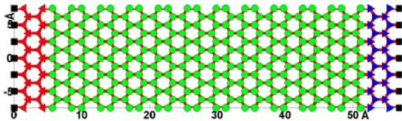
**FIGURE 1.** Rectangular armchair GNR of 1.5 nm  $\times$  5.7 nm used in this study.
