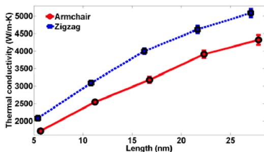
**FIGURE 5.** Thermal conductivity of rectangular GNRs with armchair (solid line) and zigzag (dashed line) long edges versus their length at 300K.
