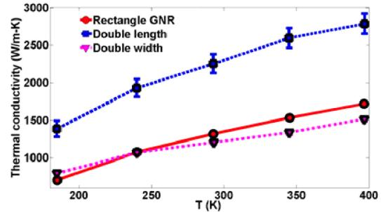
**FIGURE 4.** Thermal conductivity of the GNR in Figure 1(a) (solid line) and that of the GNR with double length (dashed line) and width (dash-dotted line) only.
